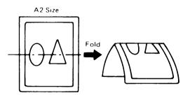
You can also transmit an original that is wider than the document guide; fold it in half and use the manual feed lever, as follows: Be sure to use Memory transmission (the Memory indicator must be lit).
